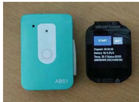
Figure 3: Wireless bio-sensor (left) and wristwatch-type information device (right).
