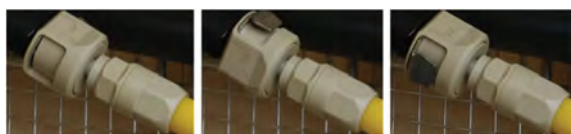
Figure 7: A variety of reference images of the same adapter because of the longitudinal rotations, which are not detectable with the feature detection algorithms.
